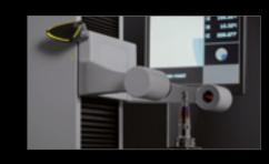
By scanning the ZOLLER »idChip« on the presetting and measuring machine, the tool data is called up directly and the measurement sequence can start.
